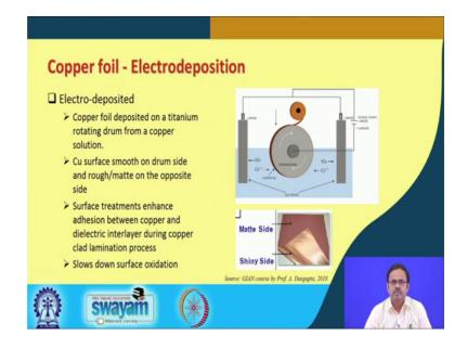
So, we are talking about copper foil. And we said that there are two different ways by which this copper foil can be made. The 1st is called electro-deposition, which is shown over here. So, what is this in electro-deposition, if the copper is electro-deposited, the copper foil is then first you have what is it is a rotating drum made of titanium ok, which is dipped in an electrolyte and then there are two electrodes ok. So, what happens is the
