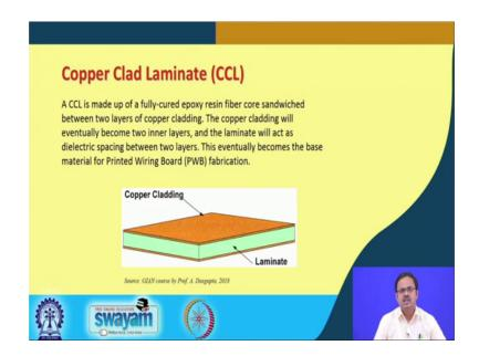
Now, this one is a very basic unit that goes to make a motherboard ok, so this is called a copper clad laminate. So, we talked about the laminate in the last lecture, what is your laminate? That is this glass you know glass, fibers or glass cloth inside this polymer matrix right criss-crossed and that is the laminate. And then, we talked about copper in the last slide.
