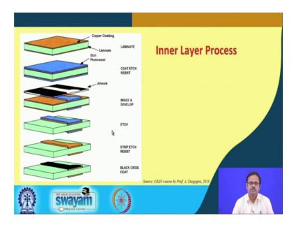
So, remember when we saw this first one this CCL copper clad laminate, what did we say, we said that these copper foils that is deposited on either side will eventually become or will eventually be the basis for having these wiring traces. We said that from this copper, we are going to retain we are going to retain that part, which is used for having these wiring traces and remove the rest ok.
