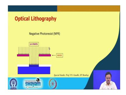
In the negative photoresist, what happens is again the same thing you have the photoresist on top that is the PDMS. Then you bring in the mask, you expose UV light and the property of the photoresist, when exposed to UV light changes, this part is till this part is the same. But, next what happens is you have some process by which the portion that part of the photoresist, which was not exposed to UV light can be removed while retaining that portion, which was exposed to UV light ok.
