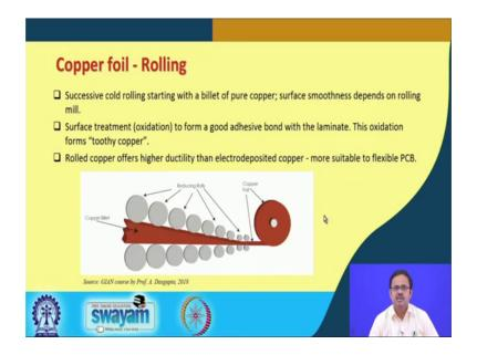
What is the other one this was an electro-deposition process, the other one is a mechanical process of the rolling ok. So, what we do is you take a thicker sheet of copper, and successively cold roll the copper. So, in the rolling mill you see, these are these rotating rolls as you see. And as a copper billet as it is called or a slab, as it goes through these rolls it is kind of thinned down.
