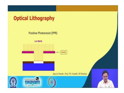
So, let us again have a recap of what we did, before when we talked about optical photo lithography. So, positive photoresist, this is my substrate. And then we have this photoresist layer, it can be PDMS for example. Then this is the mask, this is a cross section. So, as we can see the mask a lot of it is covered, and then a part of it is exposed, this is like a cutout in the mask ok. Just like your face mask, we have cut-out for eyes and nose and mouth, this is a cutout.
