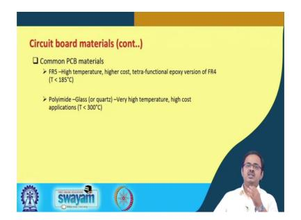
And finally, they are also two of them F R 5, this is also high temperature, high cost, tetra functional epoxy version of F R 4 ok. This can be applicable this can be applied to temperature subject to temperatures below 185 degree centigrade.
