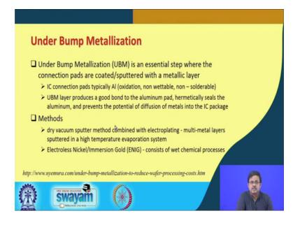
So, what is UBM in the first place? So, UBM is an essential step where the connection pads are coated or sputtered with a metallic layer. And the metallic layer is typically nickel, gold, or combination of both ok. So, it is an essential step where the connection points on the silicon is coated or spotted with a metallic layer. Now, why is it required look the connection points or the pads on the silicon are typically made of aluminum or some aluminum alloy.
