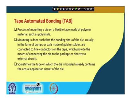
So, let us move into tape automated bonding. What is it? The tape automated bonding is a process of mounting a die on a flexible tape, made of a polymer material such as polyamide. So, here the chip carrier that we are calling or the other substrate that we have been calling so far is actually a flexible tape. And inside this tape we have these traces of interconnects going through. We will see in the pictures that will be a little more clear when we see the pictures.
