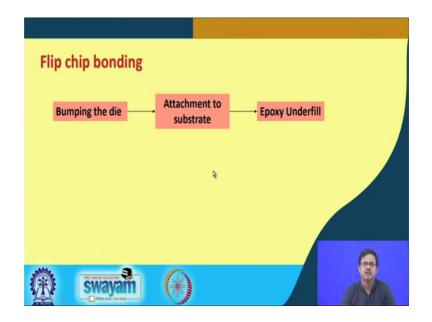
Next, what we will do is we will move onto flip chip bonding. And if you look at flip chip bonding, recall what was flip chip the active side of the die where you had this connection pads, that is flipped over ok, and then attached to the substrate alright. So, the first thing was in the and we saw that in flip chip typically most commonly, it is a ball grid array package, you have solder bumps or solder balls.
