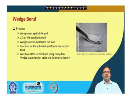
Again the process is over the wire is strong after the second bond using a clamp tear ok. And this is a picture of a wedge bond, you see it is not like a wire its first of all coming at an angle and this is how it is formed, nicely formed clear. So, this is how it is so, now what we will do is I have a couple of videos that I want to show you.
