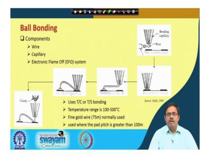
In ball bonding, these are pictures from the Wlectronic Packaging textbook by James Dally. So, for ball bonding the components that you require is definitely the wire, you need a capillary and an electronic flame off system ok. What happens? You have a
