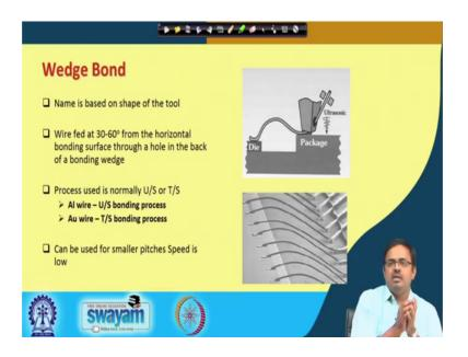
So, similarly there is something called a wedge bonding, where instead of a capillary the wedge bonding is called so, because based on the shape of the tool. So, instead of a capillary which when rises and falls, because of surface tension forces and all it gives rise to the connection or it gives rise to the shape of a like a spherical ball not exactly spherical, but it is a ball right at the connection point. In wedge bonding, what happens is you have this tool through which the wire is fed.
