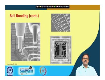
Look at this. These are actual pictures, this is actual capillary and you see how this is happening as the capillary rises this wire can be seen clear and it is called ball bonding because of the shape of this connection. Look at this shape or this shape, so that is why it is called a ball bonding ok. The previous one was a schematic previous slide pictures were schematics; these are real pictures, you can see this.
