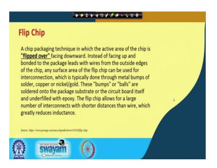
So, if we go on move on to the next slide we will start with a definition of flip chip ok. And will spend a few minutes over on this one, trying to understand what each of these term mean ok. Let us first talk about what is a flip chip ok. This is definition from PC Mag and it says that a flip chip is a chip packaging technology or a technique in which the active area of the chip is flipped over facing downwards.
