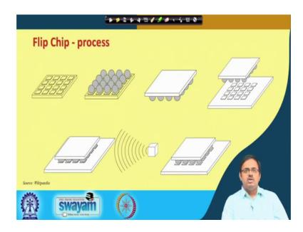
So, the next one actually is a sequence from Wikipedia. So, this is the underside of the sorry this is the piece of the chip or the microprocessor and these are all the connection points on top.
