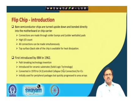
So, and talk a little bit about the introduction how it came into the into being. So, the first part is what we talked about just now again in bulletized form. Semiconductor chips are turned upside down and bonded directly onto the chip carrier or on to the motherboard.
