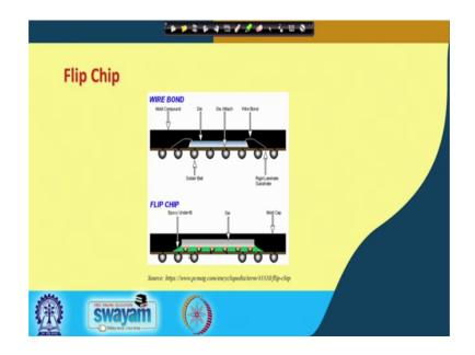
So, let us look at some of these a schematic right now and see what we are trying to say. Again this is a schematic from PC Mag and I think this picture is courtesy from m core we talked about m core technologists before. See a typical wire bond with ball grid array right is shown at the top.
