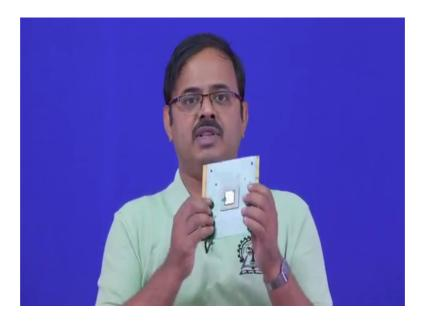
But when we talk of LGA these connections in this case pins again are also called lands are attached not on the package side, but on the motherboard side. So, that is the major difference.
