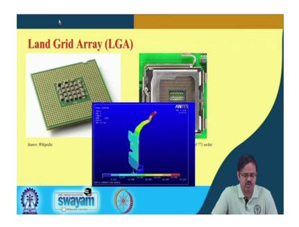
If you look at this picture it probably is a little more clear. The package side which is shown on the left what do we see? What we see there are pads on the package side these are not pins like a PGA, these are not soldered balls like a BGA. But these are just plated pads correct. And on the right hand side what you see is the socket and the socket has these pins I do not know how clear it is from this picture, but its a socket that has the pins coming out from it ok.
