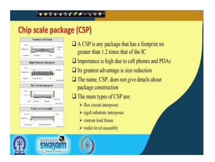
Let us move on to the next slide, this one is known as the chip scale package what is the chip scale package or CSP? We will just briefly discuss each of these a little bit. The CSP stands for a Chip Scale Package means that the size of the chip is comparable to the size of the package. The package is less than 1.2times the size of the IC.
