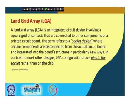
So, a land grid array this is a definition from something called technopedia let me first read this. A land grid array or LGA is an integrated circuit design involving a square grid of contacts ok. Its typically it is square it is not necessary that it has to be a square ok. These contacts that are connected to the other components of the printed circuit board; so if you look at just this first sentence, this is applicable to pin grid array this is applicable to ball grid array.
