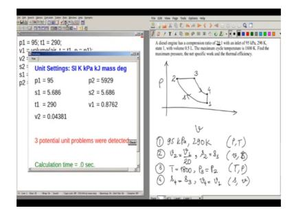
So, let us see what the pressure is; so, the pressure comes out to be approximately 5.9 mega Pascal that is a lot of pressure. So, p 3 will also be correspondingly equal to p 2 and t 3 will be also equal to 1800 Kelvin. So, then s 3 will be entropy of air at p equal to p 3 and t equal to t 3 and s 4 will be equal to s 1, v 4 will be equal to v 1.
