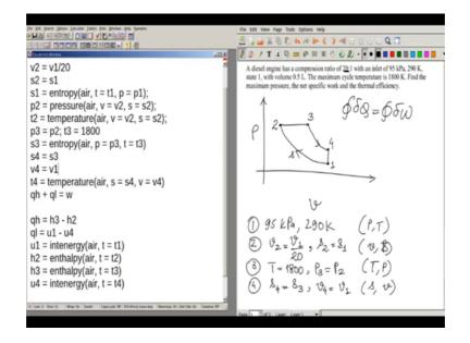
So, let us see what is wrong. So, this is the mistake s 4 is not equal to s 1 rather it is equal to s 3. So, because this is small mistake we were able to get points 4 and 1 identical ok. So, the q l is equal to minus 430. So, we already seen that we are did not account for the sign and rotate simply s q h plus q l. But, because q l is negative we understand that the process from 4 to 1 is losing heat instead of gaining heat.
