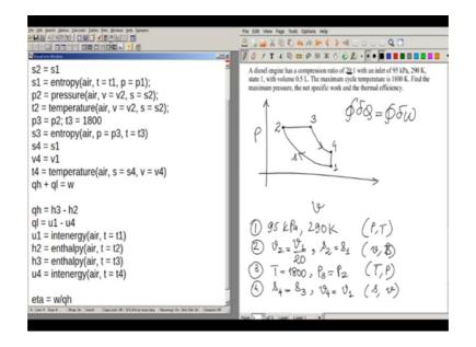
And u 4 is the; so t 4 we can find out using s 4 and v 4. So, with the help of this and the heat we have eta is equal to w by q h, this defines the thermal efficiency.
