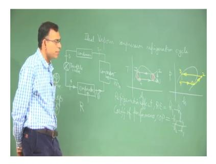
So, in a vapour compression refrigeration cycle, what we are going to study is that how we do get refrigeration? So, in the refrigeration process we see, that heat is continuously extracted from a cool place, that we make a cold place kept always cold. So, how it is possible? It is possible by this set of devices.
