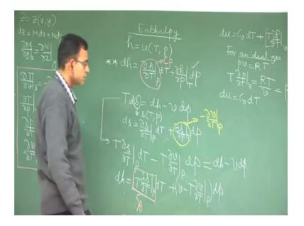
So, this is an expression now for an Ideal gas you have pv is equal to RT. So, del p del T at constant volume is equal to R by v right. So, T del p del T at constant volume is RT by T that v that is p, so this part becomes 0 p minus p. So, then du is C v d T for an ideal gas this we prove by this derivation which we assumed earlier that du equal to C v d T for an ideal gas this we now prove here, now does it so this is for an ideal gas.
