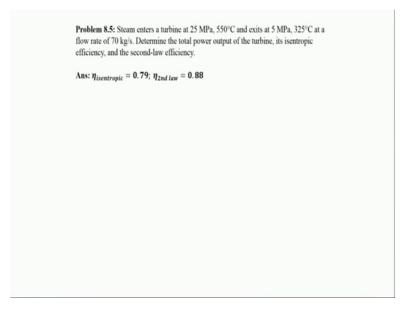
Next problem: Steam enters a turbine at 25 MPa 550 degree centigrade and exits at 5 MPa 325 degree centigrade at a flow rate of 70 kg per second determine the total power output of the turbine, its isentropic efficiency and second law efficiency. This is a very straight forward problem, but again we will try to develop an insight through this problem.
