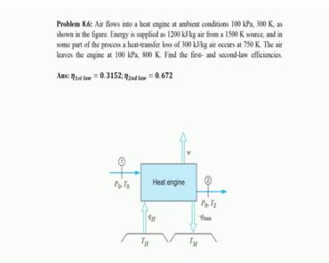
And, 300 Kelvin as shown in the figure energy is supplied as 1200 kilo joule per kg of air from a 1500 Kelvin heat source and in some part of the process the heat transfer loss of 300 kilo joule per kg of air occurs. The air leaves the heat engine at a 100 kPa 800 Kelvin find the first law efficiency and the second law efficiency.
