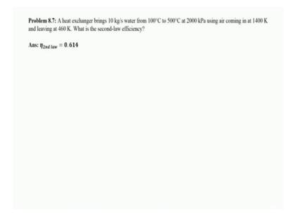
So, problem 8.7: A heat exchanger brings 10 kg per second water from 100 degree centigrade to 500 degree centigrade at 2000 kilo Pascal using air coming in at 1400 Kelvin and leaving at 460 Kelvin. What is the second law efficiency? This a very typical problem because so far we have calculated second law efficiency with by comparing work with work, but heat exchanger does not do any work. So, how do we rate its second law performance? So, we will learn that through this example.
