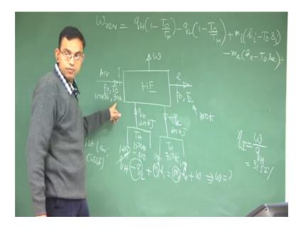
So, let us calculate this. So, you have a heat engine it is interacting with various thermal reservoir. So, you have a q H of 1200 kilo joule from T H at 1500 Kelvin, you have q minus q L which is. So, let us write this as minus q L with the magnitude of q L as 300 kilo joule. So, magnitude is 300 kilo joule minus because heat is transferred from this is what is given in the schematic of the problem. So, I am trying to be consistent with the schematic of the problem and then this T m 750 Kelvin.
