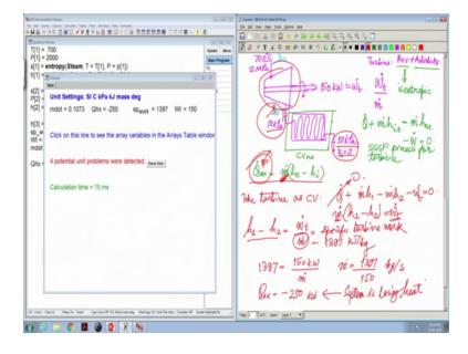
So, the heat transfer from the heat exchanger is minus 250 kilowatt, it is a huge amount of heat transfer by the way. And so the heat as per the sign convention here, the heat transferred to the system is positive and because we have a negative ones it means the system or the control volume this green control volume is losing heat. Essentially the heat exchanger is losing heat it is losing heat to take steam from state 2 to state 1. In fact, just for visualization.
