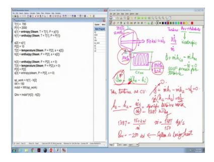
See, we know what this state is because we know the entropy and the pressure. Similarly we know what this particular state is because you know the pressure and the quality. What is not known is the mass flux? The mass flux is not known I cannot find out the heat transfer from the heat exchanger. So fine, 1397 is essentially 150 kilowatt by the
