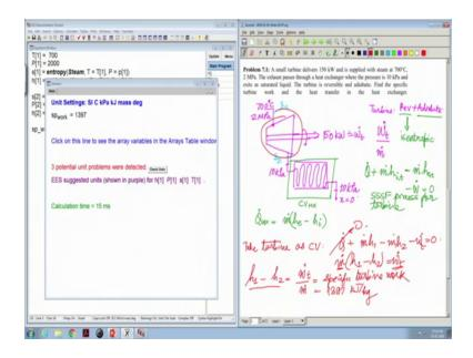
So, specific work is equal to 1397 kilo Joule per kg. Let us find out the heat transfer in the heat exchanger ok. As a matter of fact we need to find out the mass flux.
