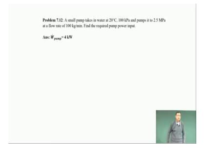
Problem 7.12, this is a sort of review problem; a small pump takes in water at 20 degree centigrade, 100 kilo Pascal and pumps it to 2.5 MegaPascal at a flow rate of 100 kg per minute. Find the pump input power input. So, the key to this problem is that it is a small pump. So, heat transfer is negligible and if you assume the pump to be reversible because no other data is given, so the work done for the pump is given by the integral v d p formula.
