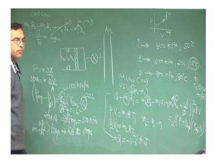
So, let me draw a schematic of this problem. This is the air supply line. There are some stops. So, what is happening is air is flowing in this line and it is supplied so that this piston expands and it might hit the stop or not from the data we have to figure out whether it hits the stops or not.
