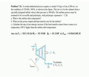
Problem number 7.11: A certain industrial process requires a supply of 0.5 kg per second of air at 200 meter per second at the condition of 150 kilo Pascal, 300 Kelvin. This air is to be exhaust from a specially designed turbine whose inlet pressure is 400kilo Pascal ok, the turbine process may be assumed to be reversible and polytropic with polytropic exponent as 1.2.
