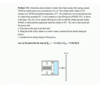
So, the next problem is problem numbers 7.10. A frictionless piston cylinder is loaded with a linear spring with a spring constant of 100 kilo Newton per meter and the piston cross sectional area is 0.1 meter square. The cylinder initial volume is 20 litre. It contains air at 200 kilo Pascal and ambient temperature 10 degree centigrade.
