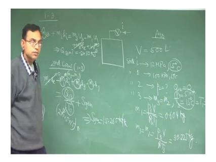
So, let us make a schematic. So, this is the tank there is a supply line with state i. So, the tank V is 500 liter state i is 12 MPa, 15 degree centigrade this is all air; state 1 100 kPa, 15 degree centigrade; state 2 you do not know p 2, but what you know is Q 12 equal to 0; state 3 at state after reaching state 2 the valve is closed.
