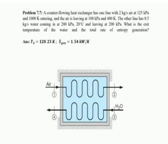
So, the next problem is problem number 7.7. So, counter-flowing heat exchanger; counter-flowing heat exchanger means that you have two streams, they are flowing in opposite directions and the heat is exchange between the hot stream and the cold stream without any external heat transfer taking place.
