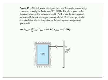
So, this problem 4.9 this is a very classical problem, this is called as a tank filling problem you know. So, what is the tank filling problem, there is a tank which is a 25 liter tank shown in the figure that is initially evacuated, it is connected by a valve to an air supply line flowing air at 20 degree centigrade 800 kilo Pascal, the valve is opened an air flows into the tank until the pressure reaches 600 kilo Pascal.
