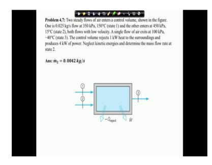
We will consider the next problem, problem 4.7. In this problem, you see two steady flows of air enter a control volume as shown in the figure. One is 0.025 kg per second at 350 kPa, 150 degree centigrade; this is state 1. And the other is 450 kPa, 15 degree centigrade, state 2. Both with low velocity; that means, you can neglect the kinetic energy of the inlet states.
