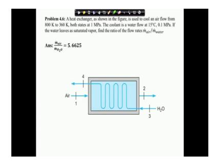
A heat exchanger as shown in the figure is used to cool an air from 800 Kelvin to 350 Kelvin, both states at 1 mega Pascal. The coolant is a water flow at 15 degree centigrade 0.1 mega Pascal. If the water leaves at saturated vapor, find the ratio of the mass flow rates? So, let us draw the schematic in the board and then we will solve the problem. This problem is very similar to the condenser problem that we solved.
