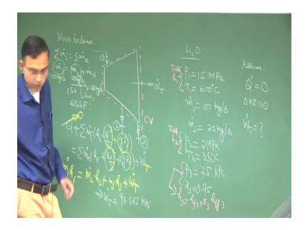
So, let us go to the board to make a schematic. So, to explain what is a steam turbine you have steam entering from a nozzle with a high kinetic energy into the turbine and it hits the turbine blades. There is a change of rate of change of moment of momentum or angular momentum that gives a net torque with respect to the axis of the turbine shaft and the turbine shaft starts rotating. So, that is how from steam power is generated.
