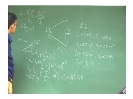
The substance air is there so you can use the ideal gas properties here, so you have pi 100 kPa. So, now what is to be obtained is what is T e and what is pe. So, we will apply the first law steady state steady flow for the diffuser controlled volume.
