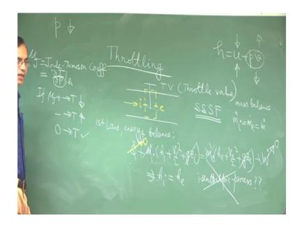
So, if mu j is positive, then temperature decreases because pressure always decrease across the throttle valve. If mu j is negative, then temperature increases and if mu j is 0, then temperature remains the same. We will show later on in one of the chapters that mu j is equal to 0 for an ideal gas and for an ideal gas therefore this corresponds to a situation where temperature before throttling is same as the temperature after throttling.
