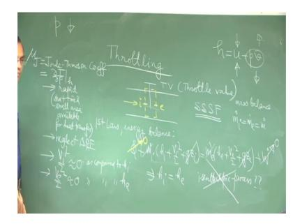
So, imagine that instead of this kind of physical situation we have a valve which we called as Throttle valve. So, these valves is operated by a screw or something like this and that is why this kind of a figure and it can come up and down. When it is screwed like this, it will come down and it will constrict the flow passage just in the way in which I do the previous figure.
