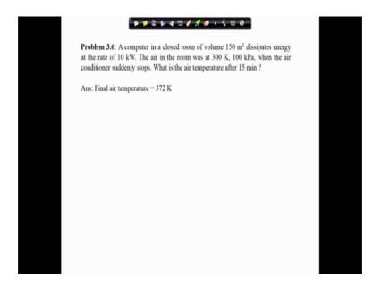
Let us look into the problem 3.6; a computer in a closed room of volume 150 meter cube dissipates energy at the rate of 10 kilowatt. The air in the room was at 300 Kelvin, 100 kilo Pascal when the air conditioner suddenly stops, what is the temperature after 15 minutes?
