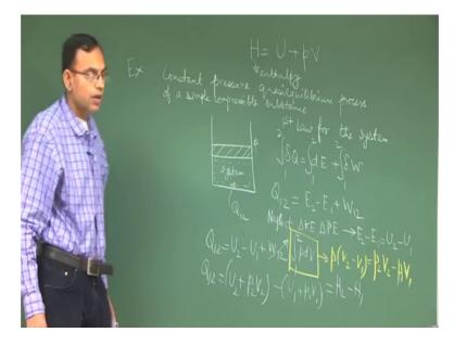
So, let us take an example of a constant pressure quasi equilibrium process. So, this is a very common example encountered in thermodynamics, where you have say a piston cylinder arrangement. There is a system here and this piston moves maybe because of heat transferred to the system Q 12, the piston moves slowly so that the pressure inside remains the same.
