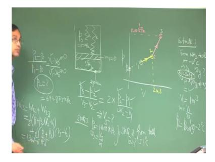
So, W 1 2 this is again a trapezium area under this. So, half into p 1 plus p 2 into V 2 minus V 1 plus half into p 2 plus p 3 into V 3 minus V 2. So, if you substitute all the values this will be 1342.6 kilo joule ok.
