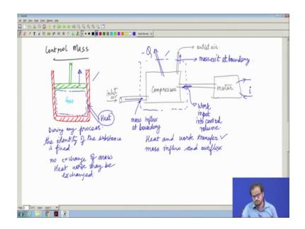
So, what is a control mass? So, very prototypical system which is used in thermodynamics is that of a piston cylinder arrangement. This is the cross section of a piston. So, this is the cylinder, this is not the piston and this is the cross section of the piston and there is some gas which is trap inside and it is assume that the piston is ideal. So, that there is no leakage ok.
