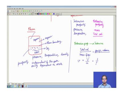
So, phase is something which has a uniform property. Let us say there is some a closed container and there is some water which is a liquid and some vapour. So, this is called to be the liquid phase, this is called to be the vapour phase ok. And, this boundary which demarcates the two is called as a phase boundary. If I heat the water the phase boundary will shift there will be more generation of vapour, the all this is common sense ok.
