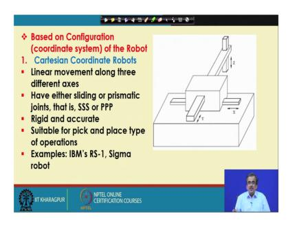
Now, here there are three linear joints. So, very easily we can imagine that the workspace for this particular the robot will be nothing but a cuboid. So, the workspace for this particular robot will be a cuboid. And this particular cuboid, I can draw this particular cuboid very easily. So, this is nothing but the cuboid and that will be the workspace for this manipulator
