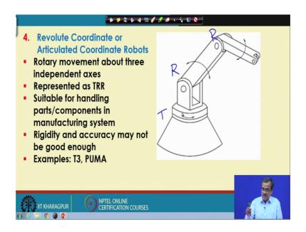
Now, I am just going to concentrate on another robot that is your the Revolute coordinate robot. So, this particular the revolute coordinate robot. Now here if I want to imagine the workspace, it is bit difficult. And as I told, we have got one twisting joint here. We have got one revolute joint here and we have got another revolute joint here.
