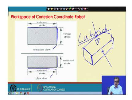
Now I am just going to find out the workspace for different types of robots. Now we have already discussed the based on the coordinate system. The robots are classified into four groups. So, we have got the Cartesian Coordinate Robot, then comes your the Cylindrical Coordinate Robot, Spherical Coordinate Robot and Revolute Coordinate Robot
