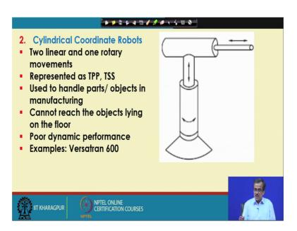
So, this is the cylindrical coordinate robot. So, as I told this is going to show me the maximum horizontal reach and the minimum horizontal reach and this will give the vertical reach and here there will be some rotation. So, corresponding to this particular your cylindrical coordinate robot. So, I am just going to imagine the workspace for this particular the manipulator
