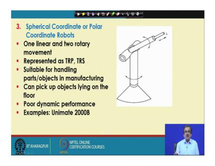
So, this is going to give the maximum the horizontal reach and the minimum horizontal reach. So, here we have got one revolute joint and here, we have got one twisting joint ok. So, I am trying to find out the like, what should be the workspace for this
