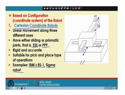
Now, the next classification is based on actually the type of the coordinate system, which is generally used. Now, based on the coordinate system we used in robots, the robots are classified into four sub groups; one is called the Cartesian coordinate robot, then we have got the cylindrical coordinate robot, then polar coordinate robot, and we have got the revolute coordinate robot.
