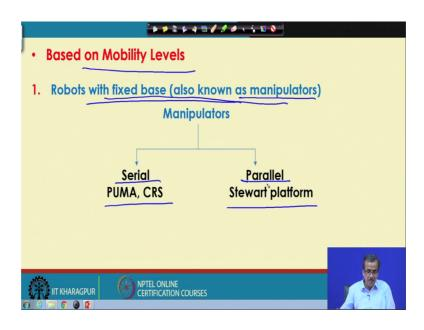
Now, another classification I am just going to discuss, and this is based on actually the mobility levels. Now, based on the mobility levels, the robots are classified into two groups, robot with fixed base, and the robot with moving base. Now, the robot with moving base, I am just going to discuss after some time.
