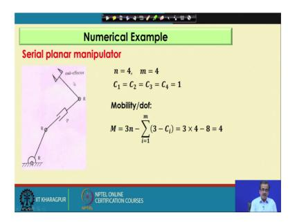
We are discussing how to use the principle of Grubler's criterion, to determine the degrees of freedom of different types of manipulator. Now, we have already seen for the serial planar manipulator. So, we got the degrees of freedom as 4. And here, this is a serial manipulator, because all the links are in series.
