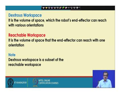
Now, if you see the dextrous workspace that is nothing but the volume of space that the robot's end-effector can reach with different combinations of the joint angles. On the other hand the reachable workspace is that volume of space that the end-effector can reach with one orientation. And this particular reachable point is was lying on the boundary of the circle.
