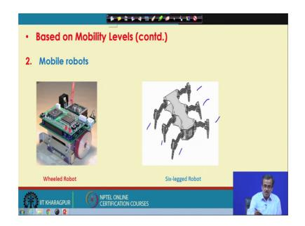
Now, here I am just going to take the example of one wheeled robot. So, this is one actually two wheeled one caster robot, it is a very simple wheeled robot. So, one wheel we can we can see here, the other wheel is on other side, and below that, there is one caster also, that is nothing but the support, so this is a typical the wheeled robot.
