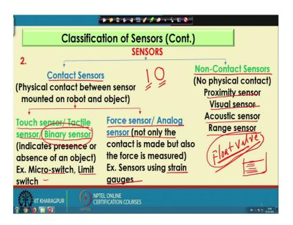
Now if you see the literature , the sensors are also classified in different ways for example, say for example, the sensors could be named as contact sensor or the non contact sensors. So, by contact sensors we mean there is a physical contact between the sensor and this particular object, whose distance I am going to measure. And if there is no such contact the physical contact between the sensor and the object that is called the non contact sensor.
