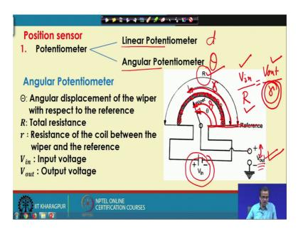
Now, I am just going to discuss one sensor one position sensor which is very frequently used in robotics or we generally use in school level, college level some laboratory classes also. This is your the potentiometer the potentiometer is actually why as I told very well known position sensor. And the potentiometer could be either the linear potentiometer or it could be angular potentiometer.
