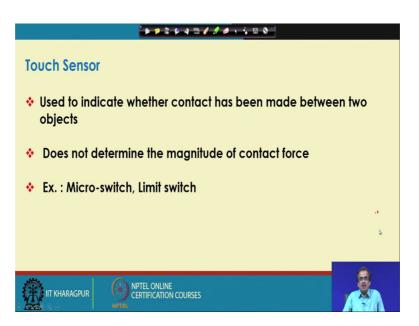
Now, I am just going to discuss the working principle of a few sensors one after another. Now this touch sensor, I have already discussed; these are use just to indicate whether the contact has been made or not. And generally we do not use this sensor to determine how much is the contact force? The examples are your micro switch, limit switch and all such things.
