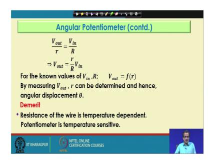
So, this is the working principle of your angular potentiometer, but this angular potentiometer has got one demerit or one drawback; all of us we know that the resistance of wire that depends on actually the temperature.
