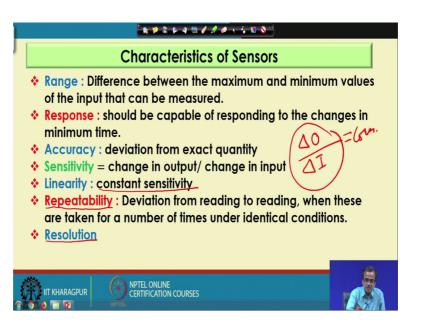
Now, before I go for the discussion of working principle of different sensors; now let me concentrate little bit the different characteristics of sensors. Like if you want to prepare the specification of sensor; so, what are the information which are to be provided and what are the numerical values to be provided?.
