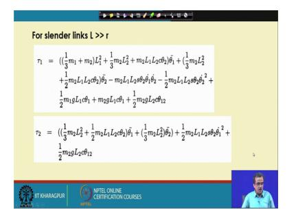
Now, we have got the expression for this particular the joint torque. And as I told once I have got the expression next task will be your how to implement in the robot in the robotic joint, so that the motor can generate this particular the joint torque which will be discussed in the next class. But before that one thing I just want to mention.
