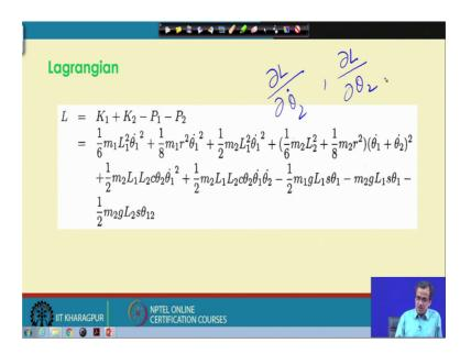
Now, we are in a position to find out the expression for this particular Lagrangian. So, this Lagrangian L is nothing but k 1 plus k 2 that is kinetic energy of the first link plus kinetic energy of the second link minus potential energy of the first link minus potential energy of the second link.
