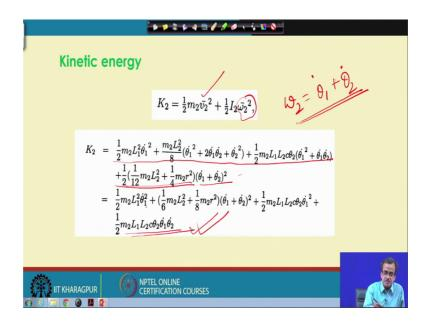
So, very easily I can find out the kinetic energy for the second link k 2 that is half m 2 v 2 square. So, I know the expression of v 2 now ok. Then I 2 I know the expression moment of inertia for the second link and this omega two, so this omega 2 will have to be careful, so this omega 2 will be nothing but theta 1 dot plus your theta 2 dot not only theta 2 dot. So, we will have to be careful.
