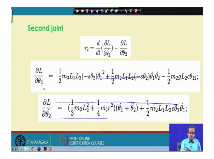
Now, let us try to find out the expression for the torque for the second joint. Now, here this tau 2 is nothing but d dt of partial derivative of Lagrangian with respect to theta 2 dot minus partial derivative of L with respect to theta 2. Now, exactly in the same way, so we will have to find out the partial derivative of L with respect to theta 2.
