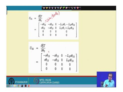
Similarly, we can also find out u 2 1 and u 2 1 is nothing but the partial derivative of t 2 with respect to 0 with respect to your theta 1. So, t 2 with respect to 0 like if you see this particular expression like t 2 with respect to 0 like your t 2 with respect to 0. So, with respect to theta 1, so we will have to find out its partial derivative.
