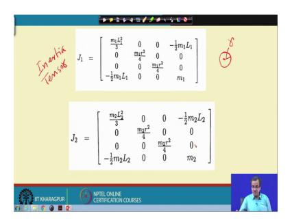
Now, if we remember you have already derive this particular expression. So, this particular j 1 is the inertia tensor for the first link. And we have consider that this particular link is having actually your circular cross section with radius r and for that will be getting the inertia tensor like this like m 1 1 1 square by  $3\ 0\ 0$  minus half m 1 1 1 0 m 1 r square by  $4\ 0\ 0\ 0\ 0$  m 1 r square by  $4\ 0\ 0\ 0$  m 1.
