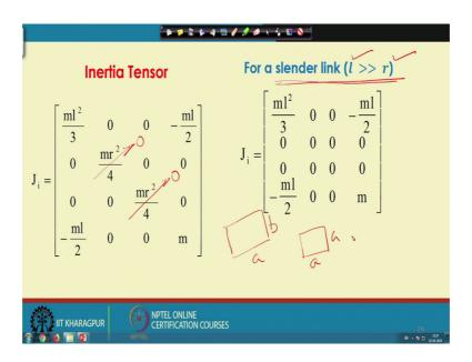
So, this inertia tensor for this particular link with circular cross section, that is denoted by J i will become equal to ml square by  $3\ 0\ 0$  minus ml by 2 then comes 0 mr square by  $4\ 0\ 0\ 0\ 0$  mr square by  $4\ 0$  minus ml by  $2\ 0\ 0$  m.
