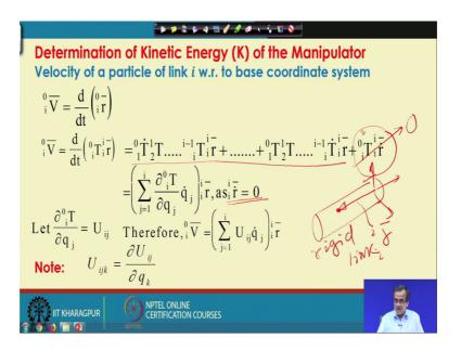
So, this r i with respect to i dot means what supposing that I have got one robotic link the rigid link something like this. Now, if this is the rigid link and I am just going to concentrate on a particular point ok. And this supposing that I have got the coordinate system here. So, this is actually the position of this particular the differential mass and this is nothing but r i with respect to i dot
