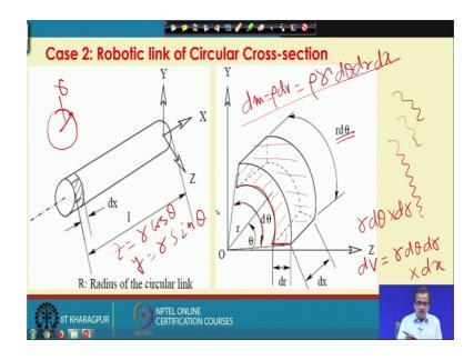
Their length of the robotic link is s into equal to 1 and it is having the circular cross section with the radius r. Now here I am just going to consider a small element, the same element I am just going to redraw here. So, this is a X Y and Z. So, the coordinate system is attached here.
