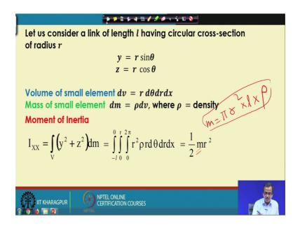
So, we can find out this and we can carry out this integration. And if we carry out this integration we will be getting half m r square, where m is nothing but the mass of this particular the link having a circular cross section. Now this mass m can be determined as pi r square multiplied by l is the volume multiplied by rho that is a density is nothing but the mass of this particular the link.
