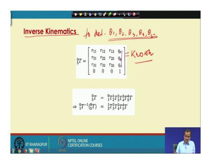
Now, let us start with the inverse kinematics of this particular the manipulator that is the mini mover. Once again the purpose is to determine the values of the joint angles like your theta 1, theta 2, theta 3, theta 4 and theta 5 provided the position and orientation of the end effector with respect to the base coordinate system those are known.
