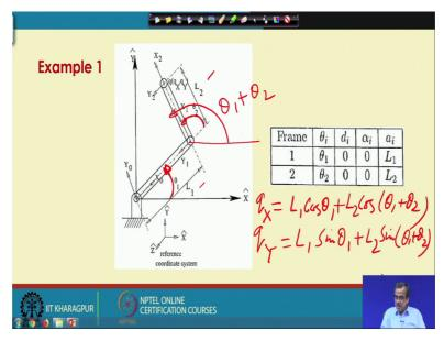
So, this is theta 1 the length of the link is your L 1 and the second link it is L 2 and with respect to these this particular joint angle is theta 2.
