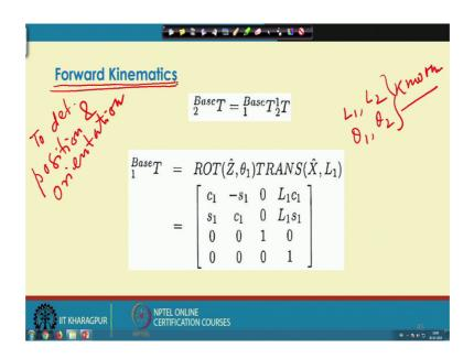
Now, in forward kinematics problem actually what we do is our aim is to determine our aim is to determine your to determine the position and orientation position and orientation of the end effector of the robot, provided the length of the links are known and the joint angles are known. So, that is actually the problem of the forward kinematics.
