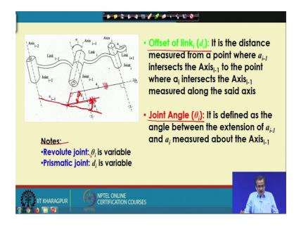
The purpose of the joint parameters I have already told that just to represent the relative position of the neighboring links. Now here there are 2 the joint the joint parameters, one is called the offset of link that is denoted by d i the link offset. And this particular link offset is nothing but the distance between the 2 points the first point is a point where a i minus 1 intersects the axis i minus 1 and another point where a i intersect the axis i minus 1.
