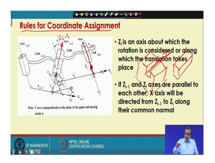
The rules for the coordinate assignment; now here we will have to find out now remember one thing, the first thing we will have to do is we will have to assign the Z coordinate system, next we try to find out the x coordinate system and after that we go for the y coordinate system.
