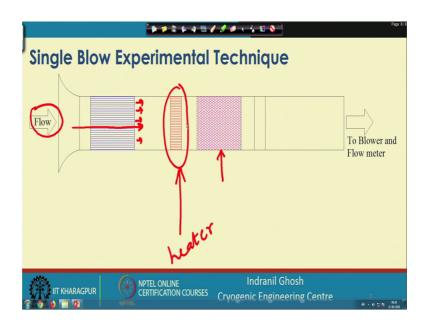
So, here we have one heater this is the heater and the when this heater is switched on. This will heat up the say if this flow is air. The air is getting streamlined and uniform with the uniform velocity, it is approaching this heater and before entering to this test section, it will get uniformly heated up.
