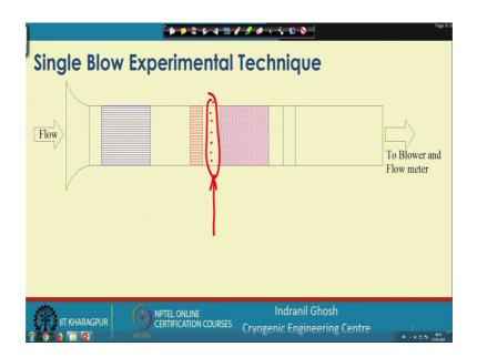
And what we do is that we have some thermocouples or the p r t, platinum resistance thermometers or some heat temperature measurement at this point. So, we measure the inlet temperature.
