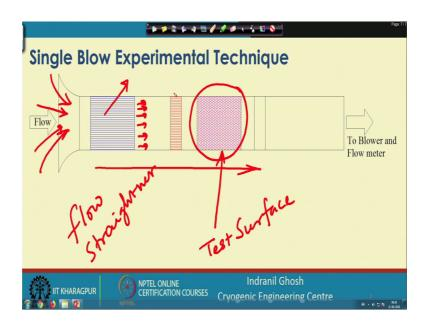
Say here, this is the typical experimental setup, where the flow takes place from this end we have the bell mouth type, of this is the flow convict through which the flow will take place this is the float straightner, this is well straight in the flow because where do with the flow is taking place from this one through this bell with this bell mouth is to the make smooth entry of the air most of the time. We use air as the fluid and here we have the flow straightner.
