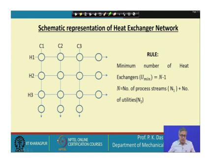
So, you see C denotes cooling stream ,and, number of cooling stream. There are three cooling streams like this and H denotes heating stream. So, there are number of heating stream like this. So, one hot stream or H 1 is to be cooled. So, H 1 is having initially a high temperature I have to bring it to a low temperature what I can do?
