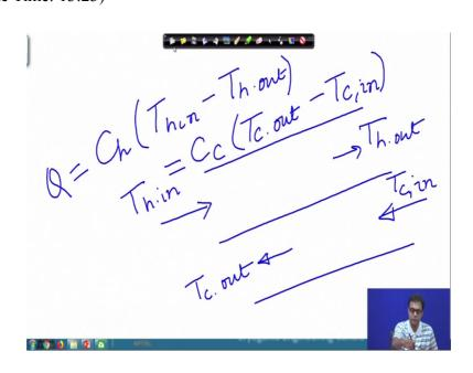
If we look again into that heat exchanger configuration; we will find that the hot fluid is changing its temperature from T h in to T h out whereas, this is T c in the counter current configuration this is T c out. So the actual heat that is getting transferred or the enthalpy change that we have said already that Q can be related as C h; T h in minus T h out.
