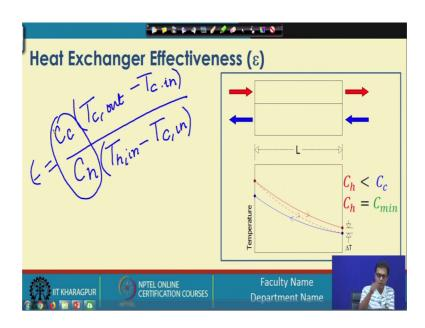
The same thing can also be written in terms of ; we can also write it in terms of the cold fluid enthalpy change. So, that becomes C c multiplied by T c out minus T c in divided by C max is Q max is equals to C h and that is equals to T h in minus T c in. We can also write this way, but this will not cancel out; so, it will remain there.
