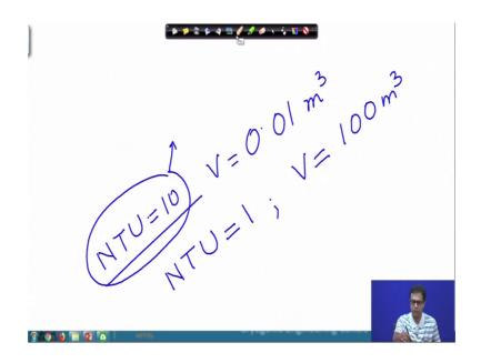
But the volume the code volume of the heat exchanger is only point 0.01 metre cube, this is corresponding to an NTU of 10. So, in another case in a chemical heat exchange chemical plant shell NTU of heat exchanger may have an NTU of 1, but it may have an overall code volume of say 100 metre cube.
