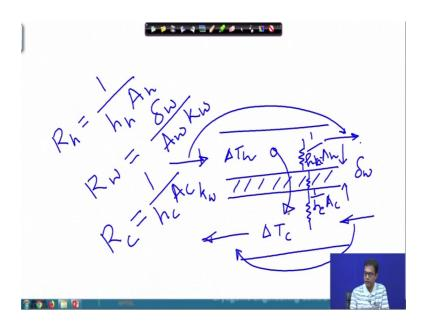
Now if we remember that we have earlier talked about a 2 fluid steam heat transfer where we had a hot fluid. And it is separated from the cold fluid by a separating wall; say this is the separating wall the thickness of the separating wall may be delta w. And its thermal conductivity may be k w and we had some hot fluid coming in and hot fluid moving out, cold fluid moving in; cold fluid moving out.
