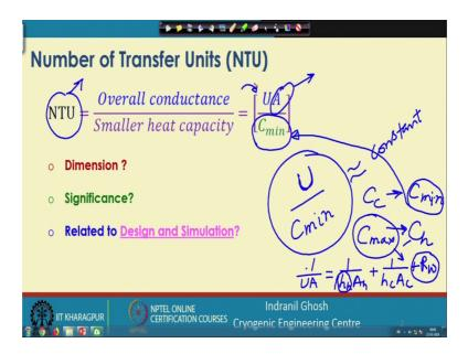
So, NTU is basically a ratio between the overall conductance and the smaller heat capacity.
