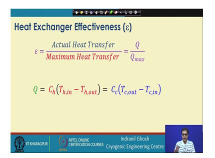
So, the effectiveness of the heat exchanger is defined as the actual heat transfer to the maximum heat that can be transferred in the heat exchanger. Now what is the actual heat that is getting transferred?
