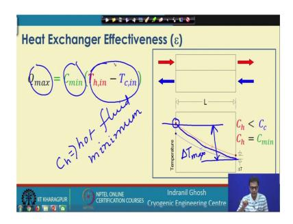
Now, if we look into here is the other situation where we have considered C h less than C c or the cold fluid is the minimum capacity sorry the hot fluid is the this is the hot fluid; the hot fluid is the minimum capacity fluid. Hot fluid by assuming C h less than C c; the hot fluid C h is the minimum capacity fluid. And that will experience the maximum difference in temperature, the temperature profile will look like this and this is the T h in.
