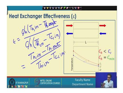
So, now if we similarly try to find out the effectiveness in other situation say in this case what is the minimum capacity fluid? C h is the minimum capacity fluid. So, if we have to now find out the heat transfer sorry the effectiveness of this heat exchanger; how can we find? We can write it as epsilon is equals to the actual heat that is getting transferred.
