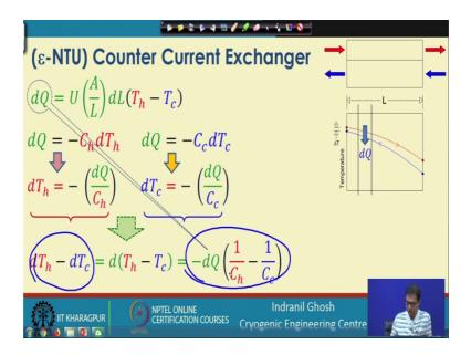
So, in an earlier discussion we have seen that in this heat exchanger; we have taken an small elemental length d L where we can write d Q; I mean in terms of the overall heat transfer coefficient or conductance multiplied by the difference in temperature.
