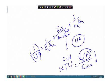
So, in a nutshell what we find that; this heat transfer from the hot to the cold fluid is limited by something which is known as the overall conductance UA or the overall heat transfer resistance UA; 1 by UA that is equals to 1 by as we have said in the earlier one this is delta w by A w, k w plus 1 by h h into A h; this is the overall heat transfer resistance or the conductance UA.
