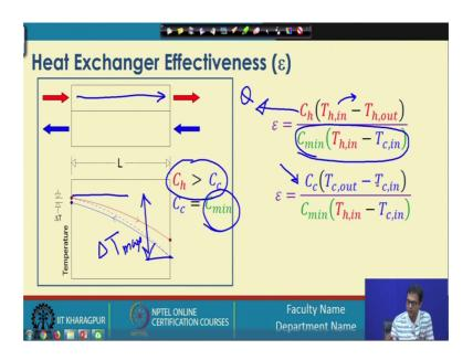
So, in case of the first situation that we have considered is C h greater than C c that is the cold fluid is the minimum capacity fluid. And in that case we can write this is nothing, but Q; Q can be written as a change in the hot fluid enthalpy change, divided by this is the maximum enthalpy that could have been changed; so C min which is C min?.
