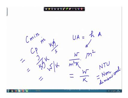
If we look at again it is individually, if we look at UA is basically nothing, but the dimension of h and A. So, this is the heat transfer coefficient that is equals to Watt per meter metre square Kelvin and this is area in metre square; so, this overall is Watt per Kelvin.
