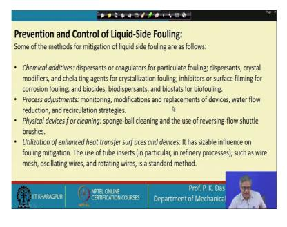
Prevention and control of liquid side fouling: Some of the methods for mitigation of liquid side fouling are as follows. Chemical additives: dispersants or coagulators for particulate fouling; dispersants crystal modifier and chela ting agents for crystallization fouling; inhibitor or a surface filming for corrosion fouling, biocides, dispersants biostats for biofouling. So, different type of fouling and what can be used.
