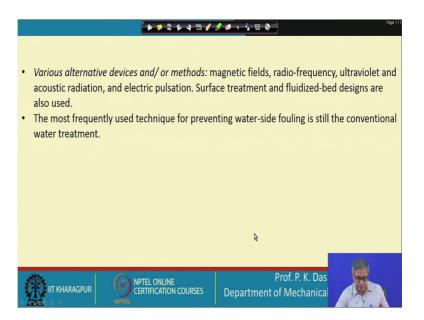
Next line slide if we see various alternative devices and methods; like magnetic field, radiofrequency, ultra-ultra violet and acoustic radiation, electric pulses and surface treatment fluidized bed design; these are all different methods. The most frequently used technique for preventing water side fouling is still the conventional water treatment. So, we had water treatment, we give treated water sometimes deionised water.
