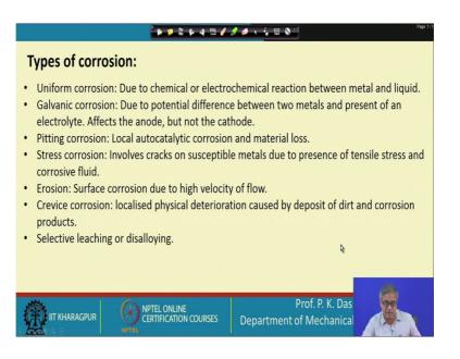
So, types of corrosion. So, there could be uniform corrosion, everywhere of the heat exchanger surface same kind of material loss is there, due to chemical and electrochemical reaction. There could be galvanic corrosion like 2 different metals are there, they do have different potential and in between there is an electrolyte. So, this forms some sort of a cell, electrolytic cell and then there is corrosion.
