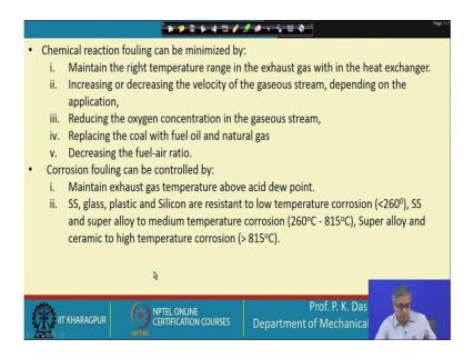
Chemical reaction fouling can be minimised by maintaining the right temperature in the exhaust gas with the exhaust gas within the heat exchanger. Increasing or decreasing the velocity of the gaseous stream depending on the application. So, sometimes we have to by increasing the velocity of stream it is convenient. Sometimes the reverse is good. Reducing the oxygen concentration in the gaseous; so many times this oxygen and
