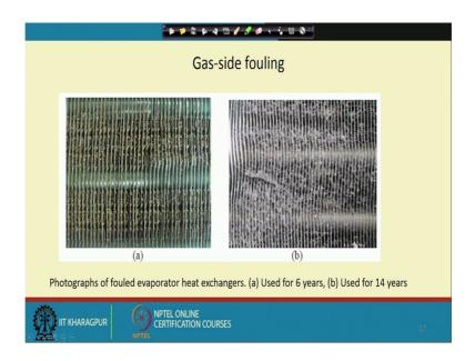
This is a gas side fouling. So, photograph of fouled evaporated heat exchanger. So, evaporated heat exchanger we can see that is it is a fin tube type heat exchanger. The tubes are visible and then there are closed spaced fins and in the fin side there will be; in the fin side there will be fouling. So, rather in this kind of heat exchanger if it if a clean refrigerant is used and there is a filter in the circulation circuit.
