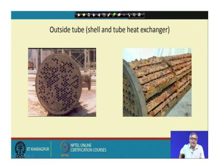
So, here I have shown the shell and tube heat exchanger; one is end view. So, this could be the tube seat in which the tubes are tubes are hold or fixed. So, you can see that in many cases, we cannot see the tube, we cannot see the area in between the tube it is so much fouled. So, obviously, here the fouling has taken place outside the tube also and here the tube bundle has been taken out of the shell.
