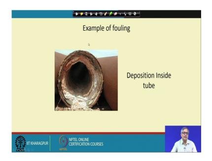
So now, I have I wanted to show some sort of fouled components of heat exchanger. So, this is a tube of a heat exchanger typical tube of a heat exchanger and you can see inside there is deposition, there is fouling and how the diameter of the tube has reduced. So, obviously, one can think that the liquid is very much fouling prone not only that proper servicing probably has not been done time to time.
