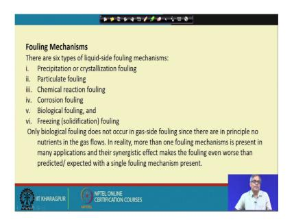
So, fouling is important. Fouling mechanism there are 6 type of liquid side fouling mechanism; precipitation or crystallization fouling. I do not need to explain it it will happen with this one some sort of chemical nature of the fluid depending on the temperature, there will be precipitation and fouling crystallization.
