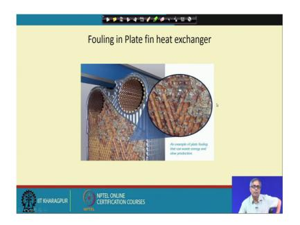
This is fouling in a plate fin heat exchanger. So, plate fin heat exchangers again plate fin; sorry, it is not a plate fin heat exchanger it is gasketed plate type heat exchanger, it is a plate heat exchanger sorry for slip of tongue. So, in the plate heat exchanger, there are small passages and plate heat exchanger should use very clean fluid because the passages are very narrow.
