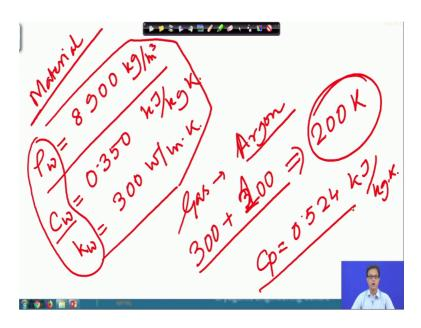
And the other parameters like say rho w that is the density is coming to be 8900 kg per metre cube this is we are talking about the copper and then specific heat C w it is also 0.350 and it is kilo joule per kg Kelvin this is the specific heat and then we have the thermal conductivity k w or k s I mean this is equals to 300 watt per metre Kelvin
