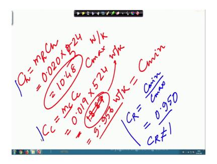
So, now we see the C h equals to m h and that will come out to be 0.02 multiplied by 524 and this comes out to be 10.48 watt per Kelvin. Similarly the C c is m C c and the mass product of this one is slightly less as we have seen this is 0.019 multiplied by 524 and this many watt per Kelvin and this comes out to be 18.87 watt per Kelvin.
