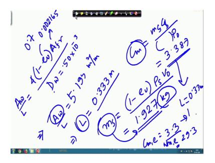
So, now, once we know the area we would be able to as we have said that we will be able to calculate the length. So, A w by L is 4 into 1 minus e v and multiplied by a frontal area divided by d w is the wire diameter.
