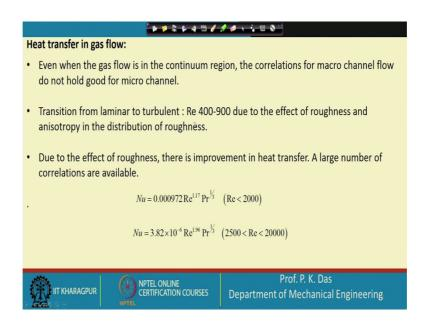
Heat transfer in gas flow and in micro channel we are considering. So, if you recall, that we have told that there could be depending on Knudsen number we can have conventional flow or continuum flow. We can have continuum flow with sleep condition at the wall, there could be transitional flow and there could be free molecular flow.
