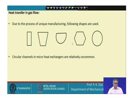
So, we have got some idea regarding micro channel. Now micro channel are modal size channel, what could be their dimension? So, that also we have some idea. What is the shape of the micro channel? The shape of the micro channels are shown here. So, you see first we can see a rectangular micro channel, then this is a kind of a trapezoidal. This is part of a circle the perception is part of a circle.
