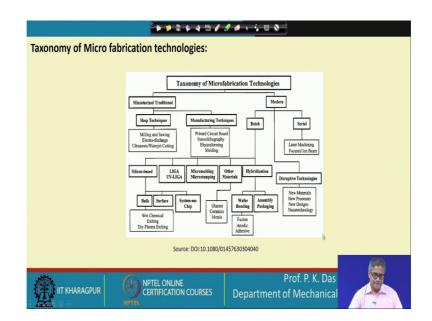
Here we are giving a taxonomy of micro fabrication technologies. Micro fabrication when I am telling or when I am mentioning micro fabrication, this is meant for making micro channels, and ultimately they can be used for micro heat exchangers. So, this is for your micro channels. Now what are the techniques? So, one side we have got traditional manufacturing, traditional method of manufacturing miniaturized channels, and the other side we have got modern method of manufacturing.
