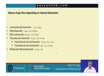
Let us go to the next information. Here all the different kind of flow phenomena has been described. And hydraulic diameter has been given in millimetre or micrometre.
