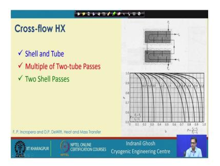
So, similarly if the geometry is changing from shell and tube, this is multiple to tube passes I mean it will be either two-tube or two-tube multiples, and there is two shell side; this is one cell side, another cell side. So, this is the expression for now this is the correction factor corresponding to that configuration.
