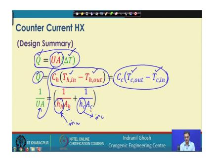
So, if we now go to the next slide so, in summary, we can say that the Q is given by UA delta T. And so, this is the final outcome we have seen, where UA is given by 1 by UA is related to the individual heat transfer I mean resistances offered by the cold and the hot fluid. And over and above, we have this individual mass balance for the hot and the cold fluid. The hot fluid mass balance is given by C h and T h in minus T h out. Similarly, for the cold fluid, we can have this equation.
