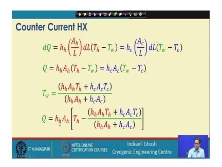
We will find that the heat transfer equation will look like, dQ is equals to as I told you that it is T h minus T w, and the area associated with this elemental length dL that is A h by L and dL is the small element and over and above h h the heat transfer coefficient of the hot fluid side. Similarly, we can equate it to the heat received from the wall to the cold fluid and the related heat transfer surface area and the heat transfer coefficient corresponding to the cold fluid side.
