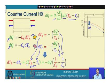
Now, in this case what we will find that the heat transfer coefficient or the overall heat transfer between the hot fluid to the cold fluid, can be related to the overall heat transfer
