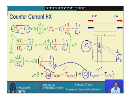
What is that form? D of d T h d T c is equals to U into A by L dL T h minus T c and 1 by C h minus C c. Now, what we are trying, we can now integrate it from this L equals to 0 to L equals to L. And when L equals to 0, the corresponding difference in temperature is
