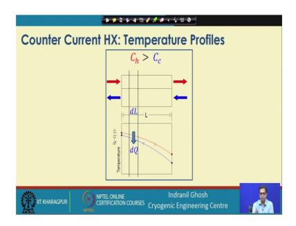
If we consider again a small elemental length dL, and then we can expect there would be a small amount of heat dQ getting transferred from the hot fluid to the cold fluid through the separating valve and all these assumptions which has been made earlier except C R equals to 1. All assumptions are still valid here, in this case also; and only exception is that we have assumed C h is greater than C c.
