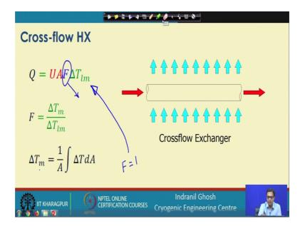
Now, if we go to the next slide, I mean if we find that there is a cross-flow heat exchanger. Do we think that still we can use this correlation, we can use this I mean relation, Q equals to UA delta T lm, but with small correction factor, because in this situation this delta T m or the min temperature or the log min temperature that is not the same.
