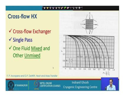
Similarly, the other configurations will be like when we have a cross-flow heat exchanger with single pass, where both fluids are unmixed or both fluids are mixed; one fluid mixed another fluid unmixed. This will correspond to a different correction factor. So, based on this values of the F factor, we have to add some correction to that LMTD method to solve the Q equals to UAF delta T lm, and then we can design the cross-flow heat exchanger.
