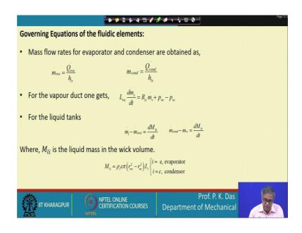
So, m dot eva that is Q dot eva divided by the latent heat. Similarly, m dot condenser that is whatever is the heat divided by the latent heat. And then there are ducts, which are the there is a duct we have conceptualized a duct, which is carrying the vapor. For that, some sort of a pipe line equation with resistance etcetera, we will get like this. For liquid in tank, we will get this kind of equation. Two liquid tank, one for evaporator, and one for condenser, we will get these two equation.
