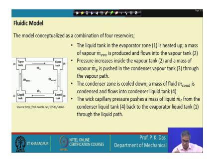
For the fluid model, the fluid model as I have told that it is a circulatory kind of a model. Vapor is generated in the condenser sorry vapor is generated in evaporator, it goes to the condenser section, it transformed into liquid, liquid comes back in the evaporator, and it gets transformed into vapor. So, we have assumed that there are two vapor tank, one vapor tank is there in the evaporator section, one vapor tank is there in the condenser section.
