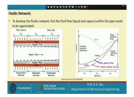
So, again we are continuing with this Heat pipes and heat exchanger. What I will do? I will go back to our previous last slide of the previous lecture, so this slide. So, fluidic network to develop the fluidic network, first the fluid flow liquid and vapour within the pipe needs to be appreciated. First, we have to understand this.
