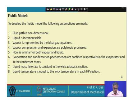
Now, if we move to the next slide, next slide means we have to go here fluidic model. To develop the fluidic model, the following assumptions are made. Fluid path is onedimensional. Liquid is incompressible. Vapour is represented by the ideal gas equation. And then vapour compression and expansion are polytropic process ok; it could be adiabatic polytropic process or some sort of polytropic process. Flow is laminar for both vapor and liquid.
