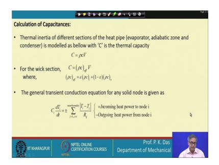
Now if we move to the next slide how can we calculate the capacitance because each of the lump or each of the node they will have some capacitance. And if we consider the transient problem then the consideration of capacitance is very important. So, basically we are talking about thermal inertia and thermal capacity. So, this C is the thermal capacity and it is given by rho C into V. Rho is the density C is the specific heat and V is the volume.
