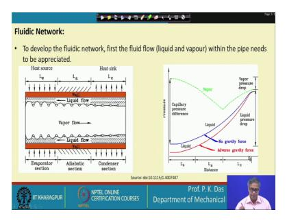
Next slide shows us the fluidic network. So, here again what we will do we will consider how the fluid flow takes place in connection with the heat pipe. I am showing on the left side and the characteristics of the fluid flow is on the right hand side and that is what we will try to consider and we will try to develop a fluidic network. First the fluid flow has to be understood and then the network has to be developed.
