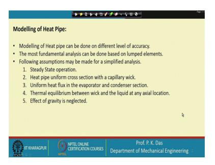
So, let me say or let me a state that the modelling of heat pipe what we are trying to do that is basically the conventional heat pipe or the most primitive and most basic heat pipe that is capillary wick supported heat pipe.
