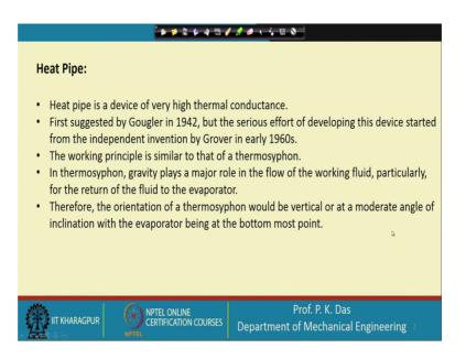
So, if we go to the next slide heat pipe. Heat pipe is a device of very high thermal conductance that is what I have told that heat pipe is a very efficient device of exchanging thermal energy. So, in general taking the heat pipe as a black box how it is doing this exchange of thermal energy that we will see later on, but if we see the heat pipe as a black box, then we can tell that heat pipe is a device of a very high thermal conductance.
