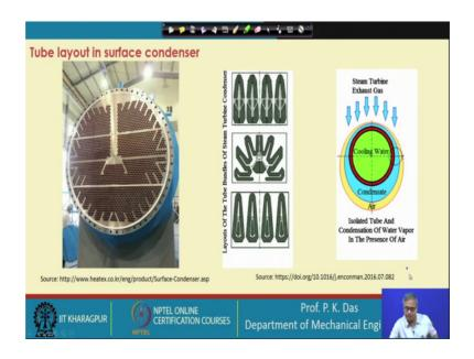
So, I am showing some sort of a typical surface condenser of a steam power plant and there are quite a few points I like to have your attention, you see this diagram which is taken from the net very carefully. So, this is showing the tube layout, first you see the tubes are laid in a very dense; configuration and the arrangement is not in line, but staggered arrangement these are all important.
