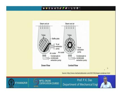
So, let us proceed here I have shown two very common situation of steam condensers and these are basically tube layout and here you see here you see, there will be some sort of some sort of greater density of cool antives. So, here we will have more cooling capacity, more vapor will be cooled and air can get separated from vapor very easily and then it will be taken out by some air extraction pump.
