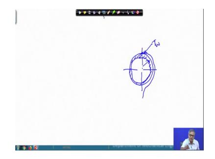
So, basically if we try to look into this problem so, basically what we are looking into let us say we have got one tube. So, this is our tube let us say some coolant is passing through the tube and the coolant is passing with sufficient velocity etcetera. So, that the outer wall temperature is kept constant this is T W so, that is kept constant this is actually TW wall so, that is kept constant.
