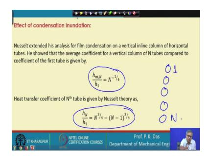
And for that what we have to do the plain analysis of Nusselt which we have done that is inadequate. So, there is one phenomena called effect of condensation in inundation, what is that? That from the top tube film is falling on the tube below it and changing it is heat transfer capability.
