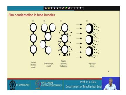
So, the effect has been shown here this is a tube row you will appreciate I have shown you the cross section of a power plant heat sorry, condenser that how many tubes are there? Very large number of tubes are there, one tube below another tube below another tube like there. So, many tubes are there.
