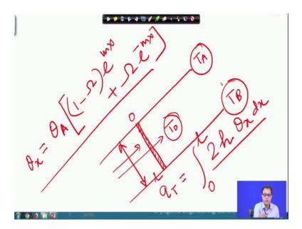
And we have derived some kind of we have obtained some kind of temperature difference or temperature profile theta x is equals to theta A multiplied by omega into to the power x, it was of this nature 1 minus omega into e to the power m x plus omega into e to the power minus m x, where omega is having a relation between r and sign hyperbolic m l.
