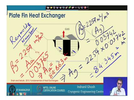
So, that is equals to the heat transfer surface area a that is say the gas side and the volume between the plate that we have now calculated just now we have calculated for this is equals to 0.03742 meter cube and it will come out to be this is beta g its a unit was sorry meter square per meter cube and this is equals to this is in meter square and this is in meter cube. So, we have a for the gas side is equals to 2254 multiplied by 54 multiplied by 0.03742.
