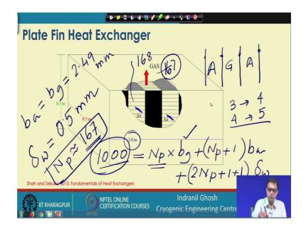
Now if we look into that then we will have N p into b g plus N p plus 1 into b a plus how many number of plates are there. If we have 2 layers of say the gas and air and say another air, so we have 1 2 3 number of streams then we have 1 plate 2 3 4 number of separating plates. So, for 3 we have 4, if we have 4 number of streams we have 5 number of plates. So, always the if we have N p plus 1 plus N p. So, it is 2 N p plus 1 number of
