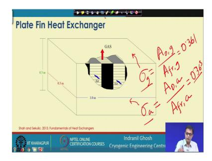
Sorry a free flow area for the gas side divided by A frontal area for the gas and similarly the sigma for A free flow area of the air side divided by A frontal area for the air side. So, this will come out to be 0.361 and this will become 0.363. These are the values for the sigma and this sigma will come as the I mean in terms of the pressure drop correlations and other correlations this becomes useful.
