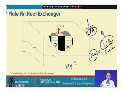
I mean this UA we are trying to calculate because that will give us, if you remember in the last class we have talked about that we intend to find out the Nusselt number sorry the Ntu, we wanted to find out and that Ntu is basically UA by C min and that UA by C min we want to calculate and for calculating the UA we are trying to you know evaluate all this numbers N p and from N p we have to find out the area and so on.
