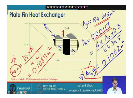
We have been able to calculate the heat transfer area and that heat transfer area for the a g is basically. A gas side was 84., the gas side has been estimated to be 84.345 meter square.
