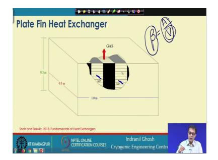
Now, we can also try to find out the volume between the plates because why this necessary because we know we have been given some parameter beta and that is has already been told about each type of fin and since we know beta we can try to find out the heat transfer area from that one, if we are able to estimate the heat exchanger area between the plates.
