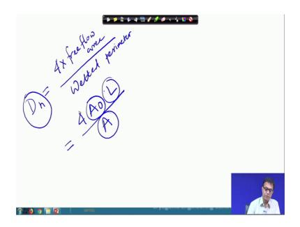
Now we know that the hydraulic diameter definition, we have written it like this the hydraulic diameter Dh is equals to 4 times the free flow area. This was the free flow area and divided by the weighted perimeter. So, we had the free flow area that was the definition we have adopted for the hydraulic diameter and this is weighted perimeter.
