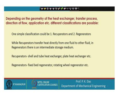
So, initially what I have told that depending on geometry of the heat exchanger, heat transfer process, direction of flow application etcetera different classifications are possible. One simple classification could be that heat exchangers can be divided into two broad classes: recuperates and regenerators. While, regenerators transfers heat directly
