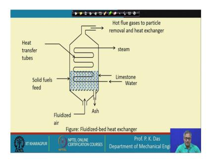
Here only one particular heat exchanger I have picked up from our last classification that is a fluidised bed heat exchanger. So, there could be different type of fluidised bed heat exchanger, but I have taken an example where in a fluidised bed heat exchanger steam is being formed from water.
