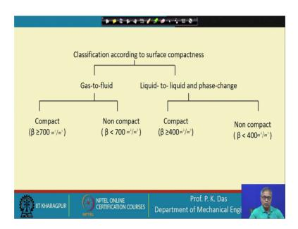
I think here we need to take some time this classification according to the surface compactness you see we will spend some time on compact heat exchanger. But compact heat exchanger this is a terminology which is used for high performance heat exchanger. The high performance could be from different aspects, but one common feature of this heat exchanger that they are having very large surface area within the given heat exchanger volume.
