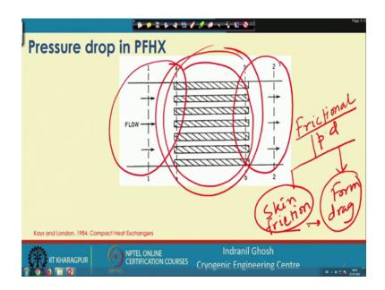
One part what we call it as the friction frictional pressure drop. This frictional pressure drop will have a 2 components one is the skin friction and skin friction and then you will have also the form dragged.
