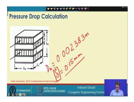
And the fin metal thickness that is delta that is equals to 0.15 meter sorry millimeter. And as you can understand that if we are using thicker fin; the pressure drop is going to be higher. And we have also be given the free flow area as well as the frontal area I mean we have already learnt about that.
