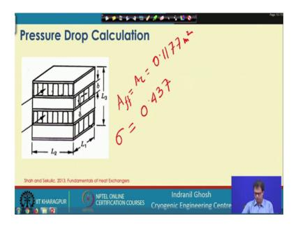
The minimum free flow area A f f or here in this one we have defined is as A f f or A c that is equals to 0.1177 then meter square. And the free flow area by the frontal area that
