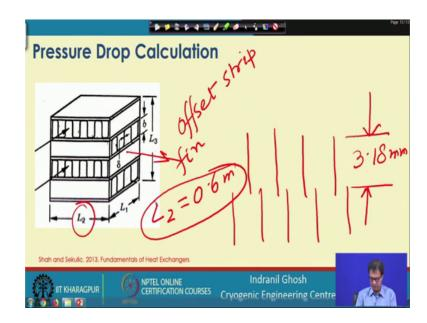
This has been given as offset strip fin and for offset strip fin we have one; if we look at this is you know this is the top view if we say. This is like we have the fin arrangement and this is what we call it as the lance length or the fin offset length; this is equals to 3.18 millimeter. And air flow length; so the air flow length L 1 this is L; L 1 or sorry this is L 2 this L 2 this L 2 is equals to 0.6 meter.
