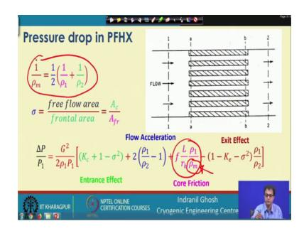
As we have told you that this sigma is the ratio between the free flow area and the frontal area and we defined it as A c by a frontal A f r. And so, most of the time we have an idea about the what is the frontal area of the heat exchanger. And we also know sometimes it is specified you will find that the sigma value will be given and from there we may have to calculate the free flow area or sometime we have the idea about the free flow area and that 2 ratio gives us the sigma value.
