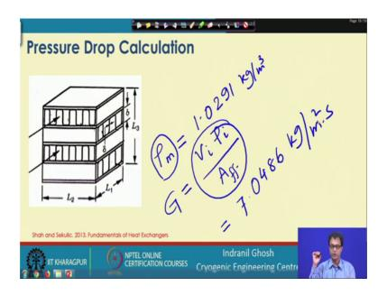
So, based on these 2 values of rho inlet and rho exit we can then calculate the rho m this will come out as 1.0291 kg per meter cube. So, this will be the main density and then we have the G; G can be estimated from the volumetric flow rate, multiplied by rho at the entry and then we have the free flow area as we have estimated that already it is given.
