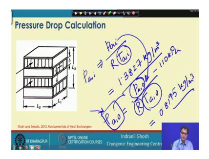
So, if we look one by one into those parameters now, if we you will find that rho of the inlet can be estimated as a function of I mean; if we assume it to be an ideal gas we can use the P v n r t relation. So, this is P air in the by R T a inlet. So, you have to convert this a into the Kelvin and accordingly this will come out as 1.3827 kg per meter cube. So, this will be the density of the air at the entry.
