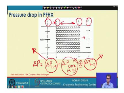
One is the core pressure drop; between this is the core pressure drop between a and b and this is if we divided it into a b and this is between a and b and this is between 1 and 2. So, we have some kind of delta P between 1 and a and then we have some kind of pressure drop in the core which will consist of we will come into that part. And there is another delta P actually here this will be a negative one and this will be minus b by b to
