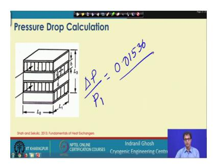
And this will come out as 0.01536. So, we can find that the pressure drop is 1.69 kilo Pascal and that is not really a very I mean it is not it is only about 1.5 percent of that total inlet pressure. So, that the assumption that has been made in our calculation that the exit pressure is not really very different from the inlet one is valid and we can.
