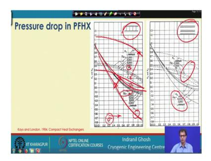
We have different K e and K c. So, not only that we have the sigma on the side we have the K e; K c values for different R e. So, depending on whether it is laminar or very turbulent where you I mean R e is infinite. So, between this limit we have the values of K e and K c; similarly we have for R e infinity at this one and the other end is the laminar one. So, between this limit this K c will vary and between this 2 limits the K c will varies for this kind of closed.
