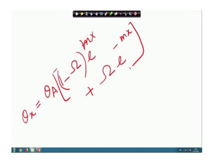
So, now if we look at we have the complete solution. Theta x is equals to theta A multiplied by 1 minus omega and that multiplied by e to the power m x, this is e to the power m x plus omega into e to the power minus m x, this what is the complete solution. Now if we have the knowledge about the fin temperature profile over the fins.
