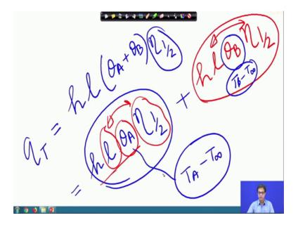
So, now, if you look at we have the heat transfer the total amount of heat transfer that q T the total amount of heat getting dissipated through the fin is h into 1 and then you have theta A plus theta B and multiplied by eta half half fin efficiency.
