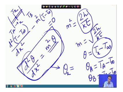
So, now if we look into this equation, we have d 2 T and we put deliberately this is the constant the fluid temperature flowing over the fin we assume at to be constant. So, we have this is minus m square and T minus T infinity is equals to 0 where this m square is nothing, but 2 h by k t are in general it is h p by k a or for thin fin thin, fin assumption this is rooted by I mean m becomes rooted by 2 h by k t.
