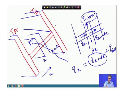
Let us look into that in details, then we have a configuration like this, we have separating walls and this is say this side is this is the fin and this fin is connected to a temperature T A and this side is connected to temperature T B.
