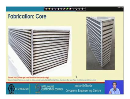
So, when we get finally, this is the kind of heat exchanger core we will get we call it heat exchanger core. So, we have only the side bars and the fins and the plates. So, it is not just, because I mean it is not like a heat exchanger, a bit this is only a heat exchanger only when we put you now the heeders on four sides or I mean different sides, it becomes it behaves like a heat exchanger.
