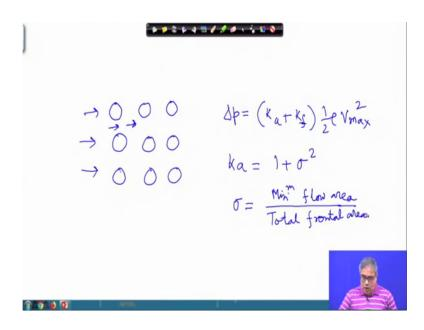
So, let us say this is the tube array, as I have told number of times that; flow of fluid is through the tube and flow of gas or air, which is the gas in many cases is in this direction. So, length of the tube is normal to the diagram I have shown. So, I have discussed the heat transfer aspect of heat, let me discuss the pressure drop aspect of heat. So, pressure drop aspect you see the when the air passes through this; it will have different cross section of area.
