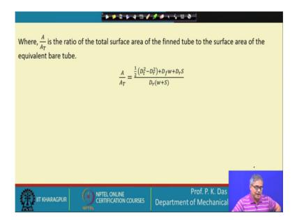
So, next slide here I have shown A by AT is the ratio of the total surface area of the finned tube to the surface area of the equivalent bare tube. So, that is what and with this we can calculate the required quantities.
