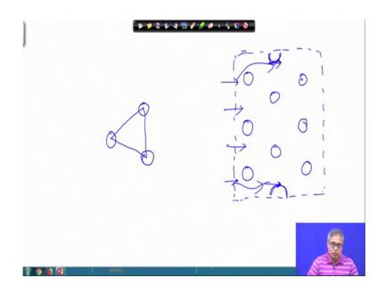
So, this is basically if we join the centre of the tubes then they are in equilateral triangular array. And then you can know that this angle this angle included angle will be 60-degree half of that angle will be 30 degree. So, this is how tubes are arranged so this is kind of a staggered arrangement. So, let us think of a staggered arrangement so this is the staggered arrangement. next row of column of tubes comes like this.
